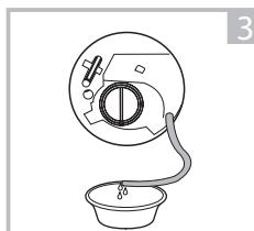
After water runs out,reset the drain hose
